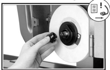
Figure 31. Barrel nut removal.
